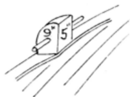
Half-Timber Head set in Plancea used as Bollard.
